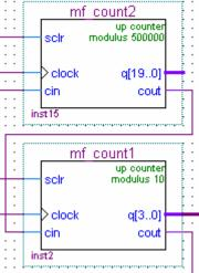
19) Lab 3.3 : Counter from elementary gates. Make a 4 bit counter that counts once a second. Construct the counter using only D flip-flops and elementary gates (ie. ANDs and XORs) according to the design discussed in class and in the homework. Use a megafunction counter to generate one carry-in pulse per second.
