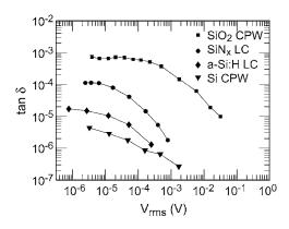
FIG. 1. Loss tangent after adjusting for the electrical loading. Data labeled SiO<sub>2</sub> and Si correspond to 300 nm plasma-enhanced chemical vapor deposition (PECVD) SiO<sub>2</sub> on single-crystal Si, and 100  $\Omega$ -cm single-crystal Si, respectively. All resonators had Al electrodes. Measurements made with  $T \leq 100$  mK.
