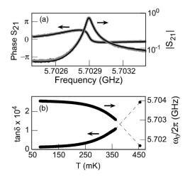
FIG. 3. (a) Measured  $S_{21}$  for an Al/100  $\Omega$ -cm Si CPW resonator (phase and magnitude, gray points) and the corresponding Lorentzian fit using Eq. (2) (black line). Resonator was measured at 86 mK with excitation  $V_{\rm rms}$  = 1 mV. (b) Temperature dependence of a resonator with the same construction as that in (a), measured with excitation  $V_{\rm rms}$ =1 mV.
