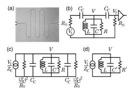
FIG. 2. (a) Micrograph of a half-wavelength CPW resonator. (b) Circuit representation and measurement lines. (c) Norton equivalent circuit  $(|Z_c| \ge R_0)$ . (d) *LCR* equivalent circuit.
