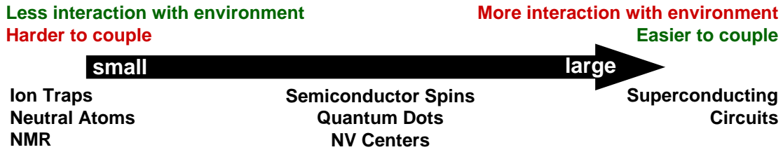
Figure 2.4: A sample of various qubit architectures. The tradeoffs among different qubit architectures are more apparent when they are grouped by physical size. Architectures with qubits of small physical size, such as ion traps, have less channels via which they can interact with their environment. As a result they have longer coherence times, but are harder to couple to each other. On the other hand, large qubits, like superconducting qubits, have more modes through which they interact with their environment. As a result, they are easier to couple, but have shorter coherence times. However, superconducting qubits have fast operation times, so compared to their smaller counterparts they are able to perform a similar number of quantum operations before they lose coherence.
