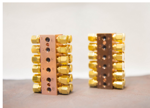
(C) Sand off the accumulated oxide for better thermal conductivity. Left: sanded. Right: not sanded.
