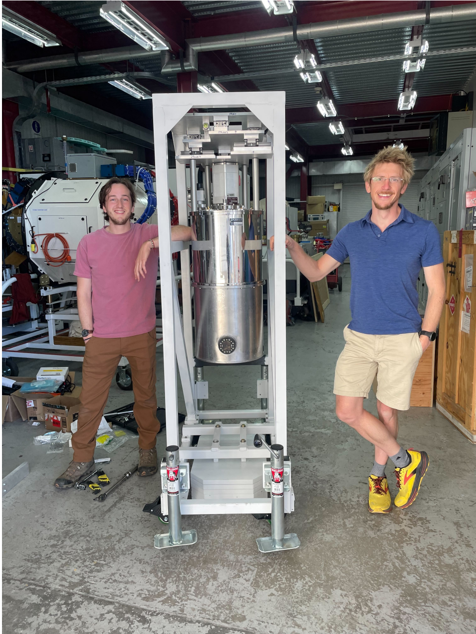
Figure 2.14 XKID mounted in its frame for the first time at LCO with Noah Swimmer (myself, left) and Jeb Bailey (right). The base can be seen at the bottom on its casters with the front lifting jacks visible. The ballast is the large mass held up by the cross beams attached to the base. The frame is the tall white vertical structure, and the linear motion control assembly is mounted at the top, which the cryostat is hanging from.
