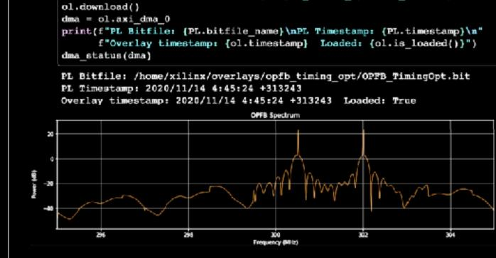
Suite of test overlays used to verify individual IP. Python drivers allow simplified interacting with the FPGA through Python.
