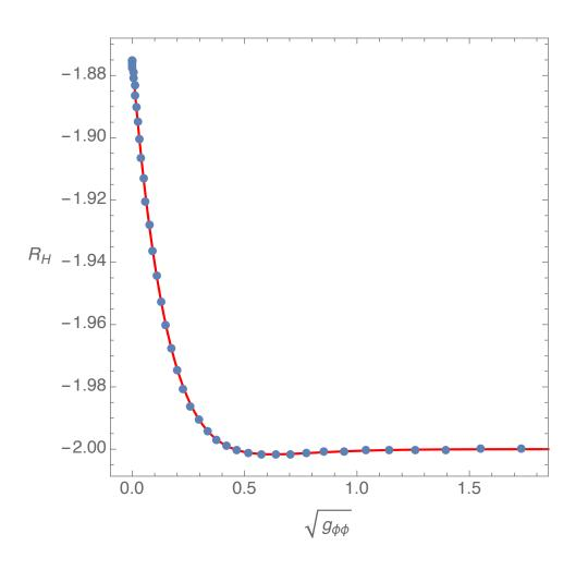
Red line is analytic solution from point charge. Blue dots are numerical data for M1 with a = .2 The charge density is now a smooth function, and again falls off like  $1/r^3$ .
