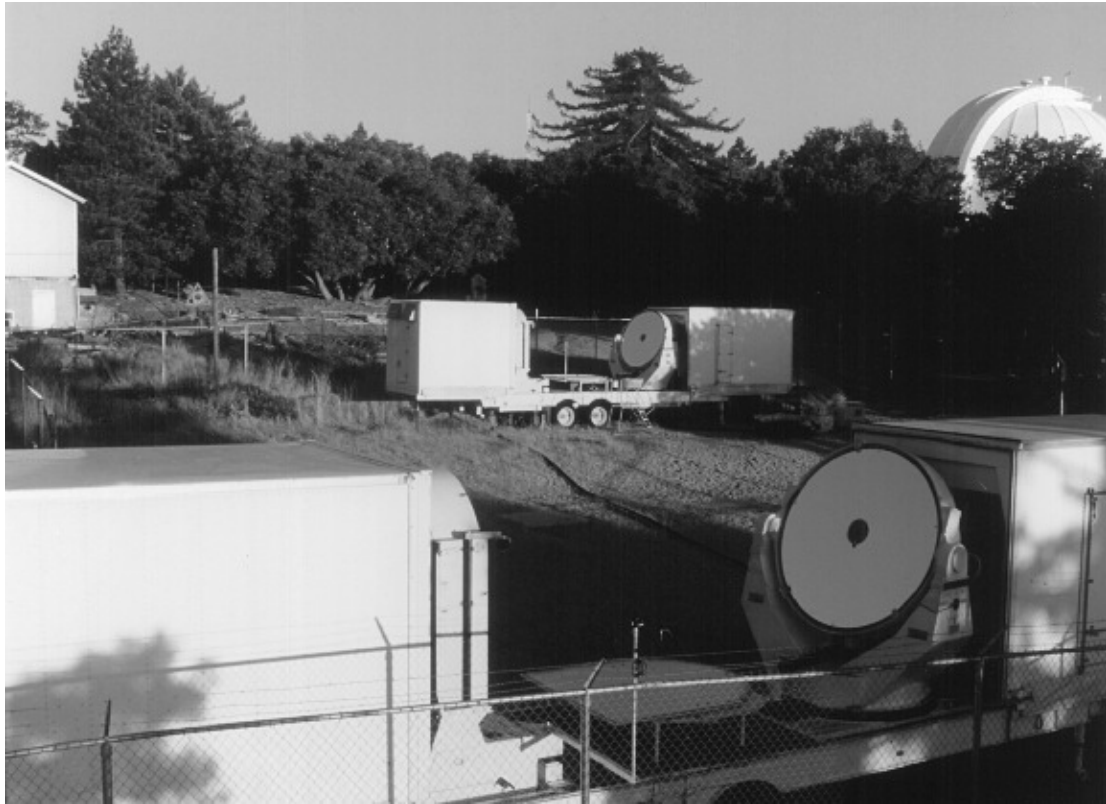
Figure 3.1: The U.C. Berkeley Infrared Spatial Interferometer. The interferometer is comprised of two Pfund telescopes, each mounted in a standard semitrailer. Here the interferometer is shown on a 32 m baseline. The 2 m steerable flat mirrors can be seen in this view. In the upper right of the photograph is the 100 inch telescope dome, where Michelson and Pease carried out the first successful measurement of the angular diameter of a star, and in the upper left is the building where a subsequent attempt at interferometry with longer baselines was made (§2.1).
