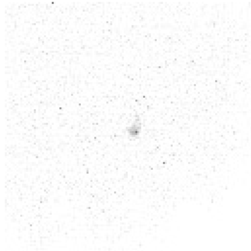
Figure 3.20: Background-subtracted guider camera image of an m_K = 3 star. The star is at the center of the field of view. This image illustrates the flickering pixels and non-uniformity which the guider can mistake for a star. Figure 3.21 shows a histogram of the data from this image. Color has been reversed for clarity. The integration time was 138 ms.
