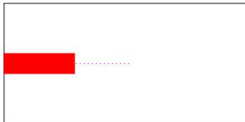
When the laser fires a pulse of light, the light is near the left end and pressure from this light pushes the box to the left. The box moves to the left while the pulse is traveling to the right. Then, when the pulse hits the far wall, its pressure stops the motion of the box. The light itself is absorbed by the wall and disappears.
