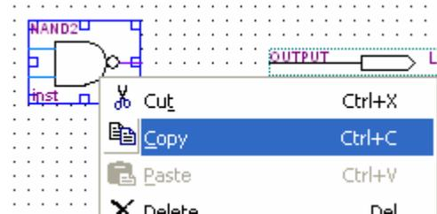
16) Make an OR gate from multiple NAND gates. You may copy the NAND gate by right clicking the gate, and using the copy and paste commands. You may also move the gates and input/output pins by dragging, or box-selecting and dragging the objects.
