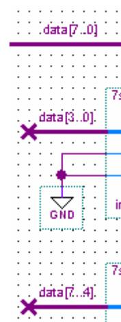
23) Compile and program the FPGA. Cycle through the numbers 0 through F on the DIP switches, and test for proper decoding of the hex into the LED display segments. Note that you will find 3 errors in the coding, which we will now fix.
