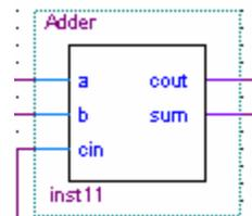
33) Complete the wiring for the 4 bits of the adder stage. Note how the a[3..0] and b[3..0] inputs are set by the dipswitch, and are broken out into the individual bit stages of the adder by naming wires. Also note the output 7 segment displays. The leftmost 7-segment display is a[3..0], the 3<sup>rd</sup> display is b[3..0], and rightmost is sum[3..0].
