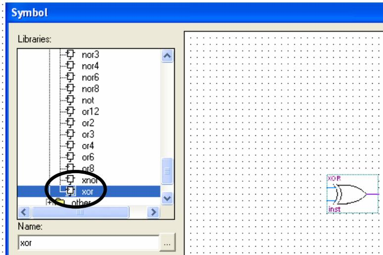
29) Wire up the gates according to Fig. 8.7B. Note that we have to break out the individual bits of the inputs to connect them to the XOR gates, but we have to get them grouped back into a bus to use the 7 segment display. This is done by naming wires and buses as we saw in the last lab. Also note how the raw input bits are grouped into a bus and connected to the LED[3..0].
