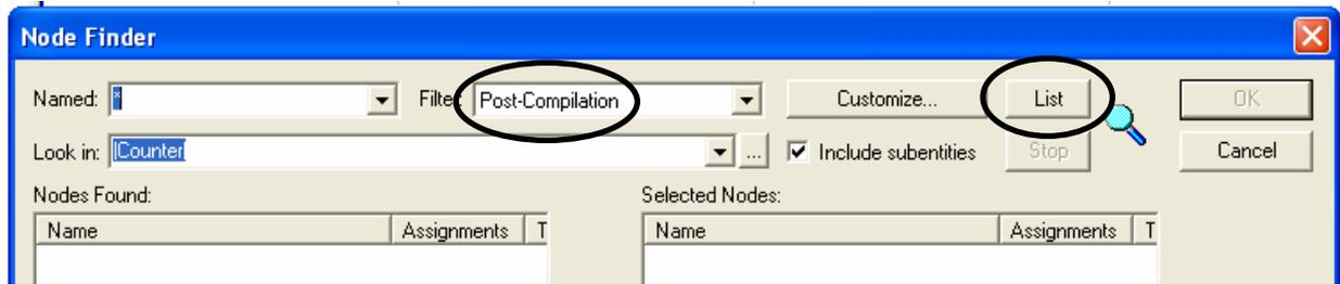
8) Double click on the nodes you want to simulate and they will move to the right hand column. Choose the inputs “fclk”, “SW\_USER[1]”, and “SW\_USER[0]”; and the output bus “DIG5\_SEG”. We have chosen the inputs as individual lines, not buses, to have separate control of the two inputs. We have chosen the output to be a bus because we want to look the entire based output. Click “ok” twice to close the node finder window and add the nodes to the .vwf file.
