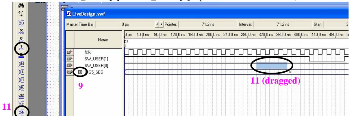
symbol to set their value to 1 for all time. Next, right click and drag over one of these waveforms to select a span of time (“dragged” above fig.). This selected time span can be set to zero by then clicking the “0” symbol. Note that the other useful input functions are invert, which inverts a selected node, and ‘c’, which increments a bus value at each clock cycle.
