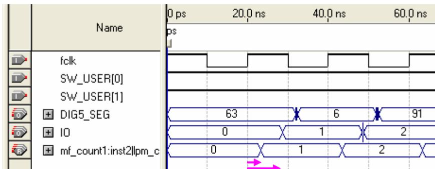
17) **Lab 3.2 : Binary-coded decimal counter.** Copy your entire folder for lab3.1 to a new folder named lab3.2. In this lab you will design a counter that displays the count in base-10 (binary-coded decimal) numbers. Make the rightmost digit of the display count in 1/100 of a second, and display a decimal point after the first two digits.
