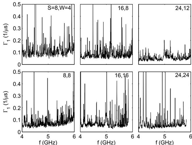
FIG. S3: Frequency dependence of  $\Gamma_1$  for six qubits with different  $S$  and  $W$ . The frequency stepsize is 5 MHz for  $S, W = 8, 4 \mu\text{m}$  and 2 MHz otherwise.
