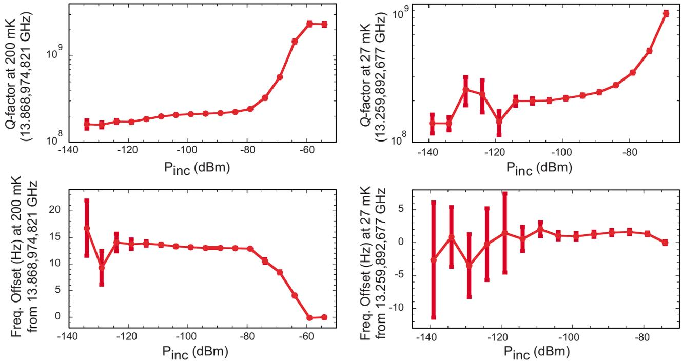
FIG. 2. (Color online)  $Q$ -factor and frequency shift as a function of incident power for the  $WGH_{20,0,0}$  and  $WGH_{19,0,0}$  modes at 200 mK and 27 mK, respectively, (as labeled).
