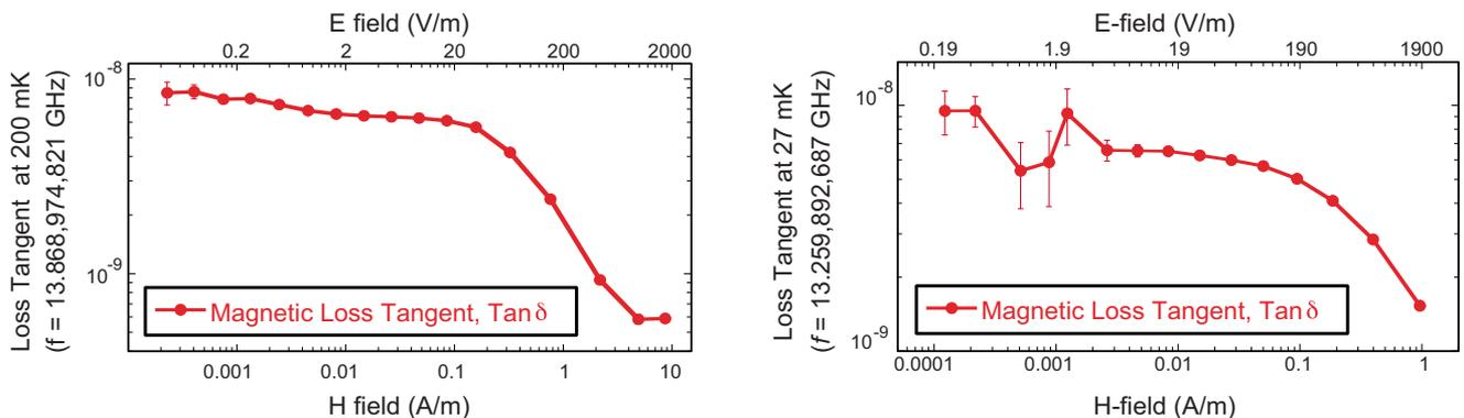
FIG. 3. (Color online) Measured loss tangent vs the  $\vec{E}$  and  $\vec{H}$  field amplitudes for the  $WGH_{20,0,0}$  mode (left) and  $WGH_{19,0,0}$  mode (right).
