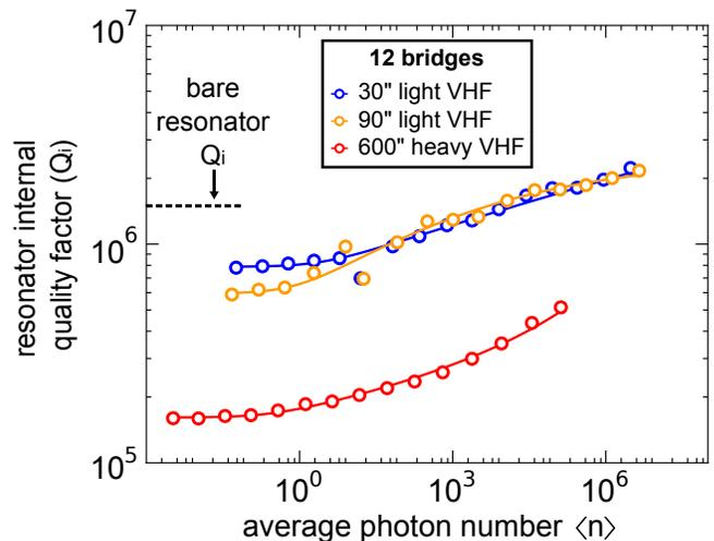
Figure 3. Representative resonator  $Q_i$  measurements for differing amounts of VHF treatment. The bare resonator has no bridges, but did receive 30 seconds of the light VHF treatment detailed in the main paper.
