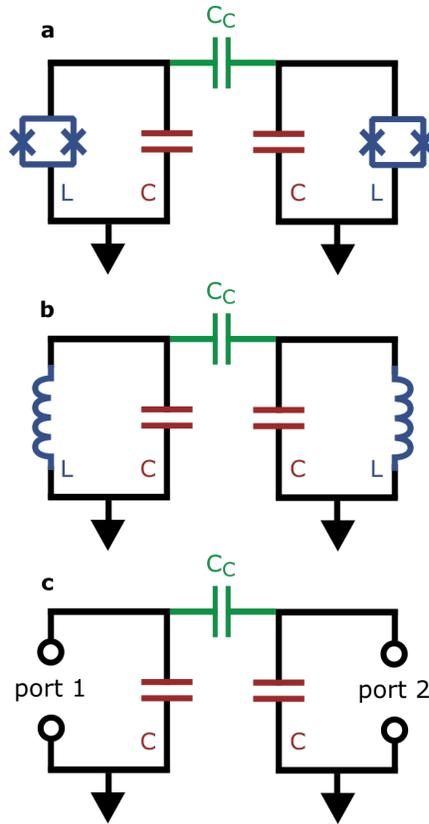
Figure 1.2: **Coupling qubits.** **a** Fixed capacitive coupling between two qubits. **b** The coupling between the two qubits can be understood (approximately) by replacing the junctions with inductors. **c** Replacing the inductors with ports allows us to construct the capacitance matrix and find the normal modes of the circuit.
