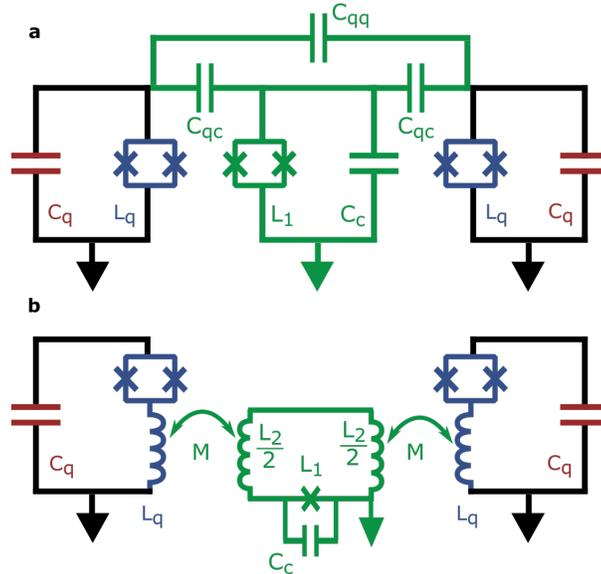
Figure 8.1: **Coupling qubits.** Two implementations of tunable coupling. **a** Tunable capacitive coupling. **b** Tunable inductive coupling. Note that  $L_q$  refers to the series inductance of the qubit junctions and linear inductance. In both cases, the coupling is controlled by an applied flux which tunes the effective junction inductance of the coupler.
