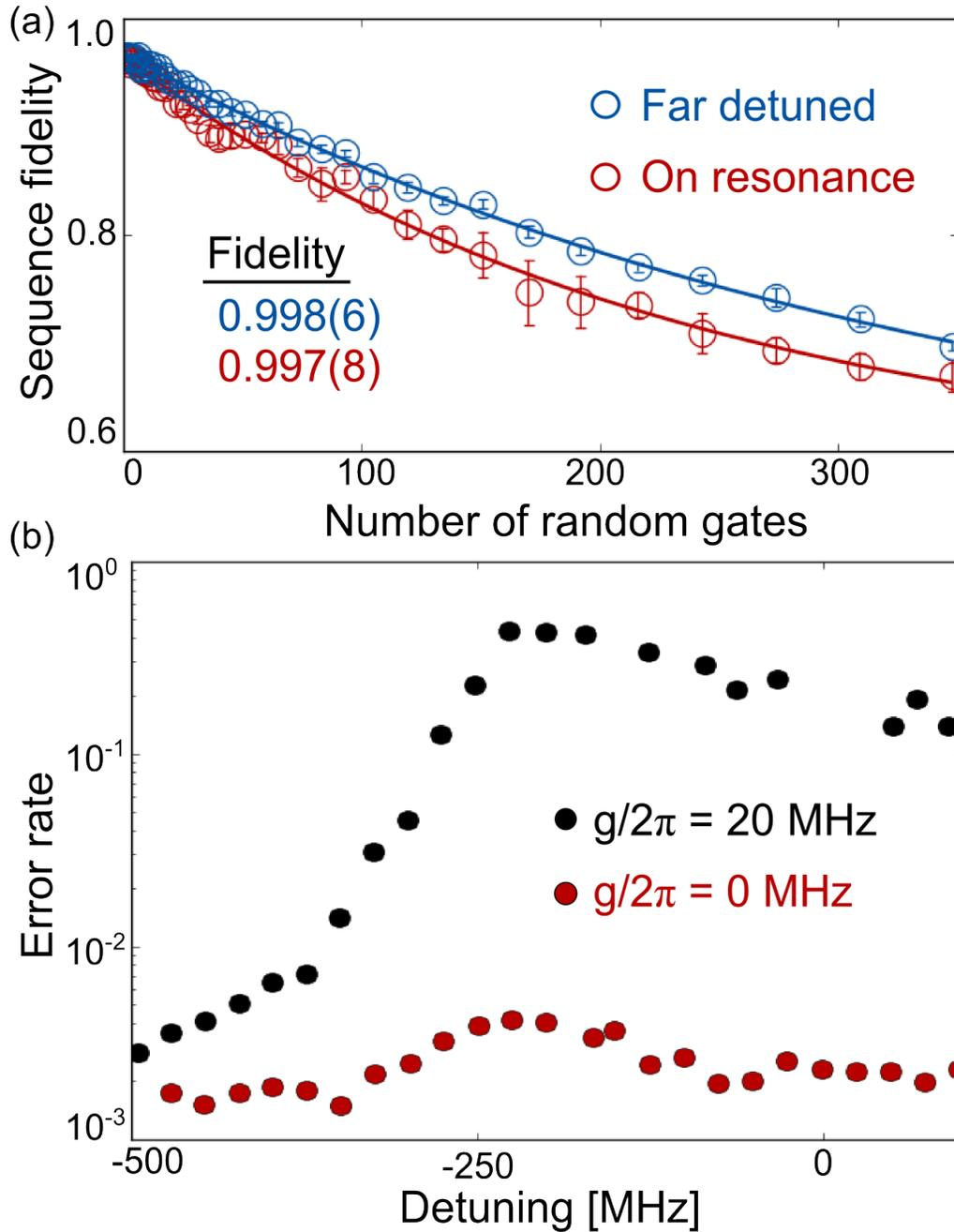
Figure 2.3: Simultaneous single-qubit randomized benchmarking. (a) Raw benchmarking data for  $Q_1$  when  $Q_2$  is far detuned (blue) and on resonance (red) with random gates applied to both qubits. Operating the qubits on resonance degrades the gate performance by  $< .1\%$ . Lines are fits to a decaying exponential. (b) The average error rate for  $Q_1$  as a function of detuning between the two qubits, shown for nominally zero (red) and 20 MHz (black) coupling.
