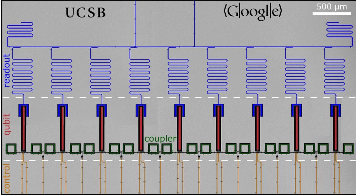
Figure 7.1: **Device: nine-qubit array.** Optical micrograph of the device. Gray regions are aluminum, dark regions are where the aluminum has been etched away to define features. Colors have been added to distinguish readout circuitry, qubits, couplers and control wiring.
