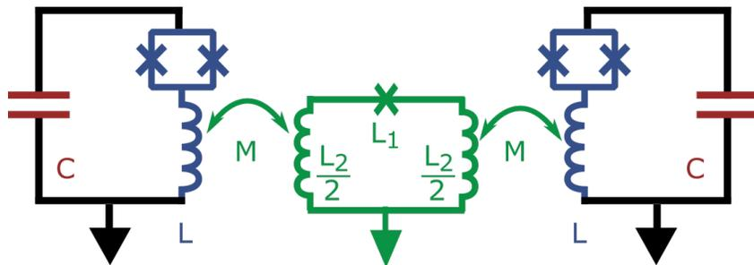
Figure 1.3: **Tunable inductive coupling.** Circuit diagram for two inductively coupled qubits. The coupling can be controlled by applying a flux to the coupler (green) which tunes the effective junction inductance.
