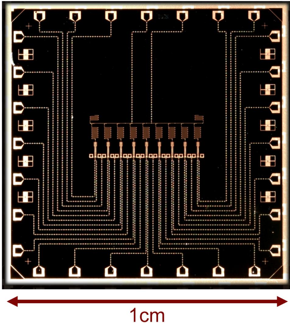
Figure E.1: An optical micrograph of the device used in this work. The chip consist of 9 qubits in a 1D chain with adjustable coupling between every pair of qubits. The qubits appear as small vertical rectangles in the middle of the chip. The couplers are the two square loops that are between the qubits. The wiring lines that are routed to the perimeter of the chip are used to control the qubits and the interaction between them. The meandering lines above the qubits are the readout resonators.
