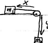
$f = x + y = \text{const.}$  (constraint)
