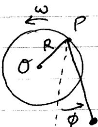
The position of P with respect to the origin O is  $(R \cos \omega t, R \sin \omega t)$
