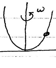
$z = K\rho^2$ . It is easiest to use cylindrical coord  $(\rho, \phi, z)$ . The potential energy is:
