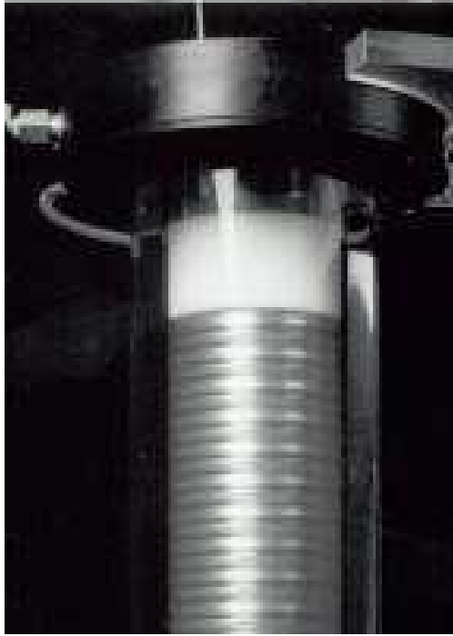
FIG. 5: A photograph of a portion of the apparatus with Taylor vortices present..
