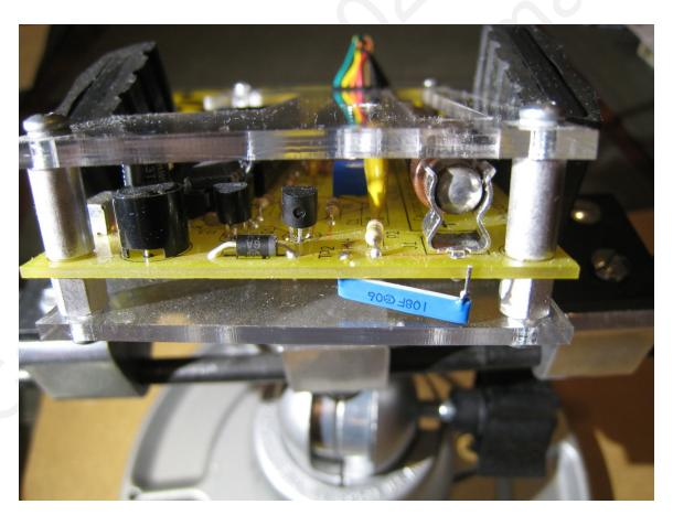
To measure the tube voltage, set a multimeter with  $10~M\Omega$  input impedance to measure DC volts, then place the positive probe on the unconnected lead of the  $1~G\Omega$  resistor, and the negative probe on the clip holding the far end of the Geiger tube. Figure out how to calculate the voltage at the HV+ test point from the meter reading. The tolerance of the
