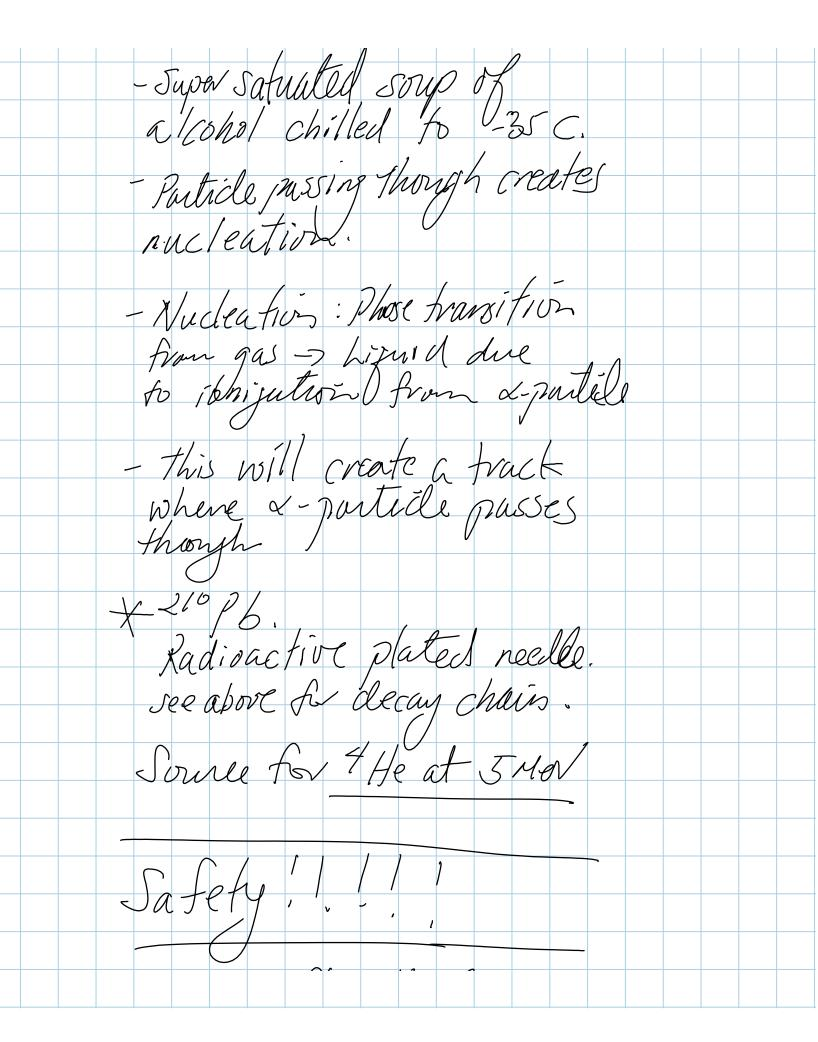
Alcohols: flammable & Toxic. Not the drinkin kind! Power on Coslin before the Chumber. Compressed Gus = Dongerows. Gas escape though top hole of the chamber. Gas is an asphyxiant. Do not run confinously Open door it redded Close cylinder vulve at the send of use.
