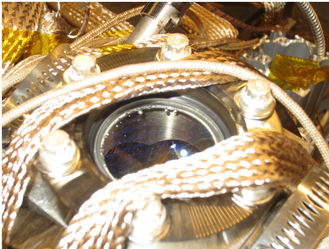
Figure B.2: A photograph showing the source of the failure in our first attempted Li oven bake. The glass-to-metal seal was heated above its rating, leading to the sealant melting. This was caused by non-uniform heating due to direct heating of the chamber.
