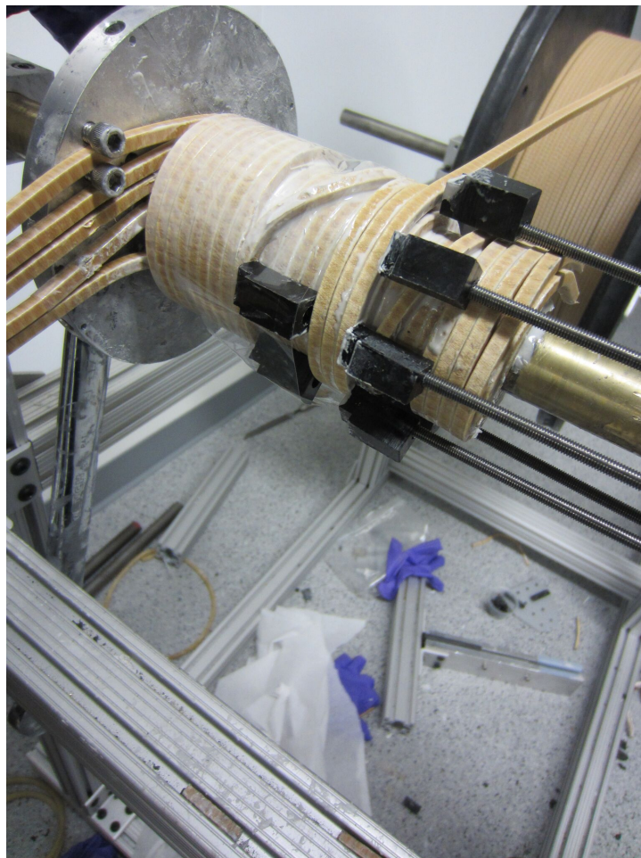
Figure 5.11: A photograph taken midway through the slower winding process. This photograph was taken after the completion of the fifth layer of the same slower segment as shown in Figure 5.10. Note the implementation of a gap between coils in this layer.
