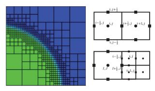
**Fig. 3** Numerical discretization: a typical spatial discretization employed during the simulations to resolve a bilayer domain (left). The Cahn–Hilliard equations are discretized using a finite volume numerical method with fluxes represented on the faces of the control volumes and the phase field *c* represented in the centers of the control volumes (right).
