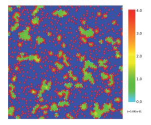
**Fig. 8** Simulation snapshot at  $t/t_{max} \approx 0.6$ . Some initial SLB domain merging has occurred, but individual bilayer islands are still present. We see that island sizes stay within our estimated bounds of between 3 and 10 vesicle radii.
