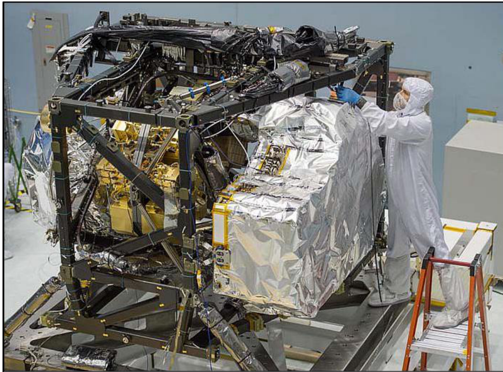
The JWST ISIM is shown in final preparation for thermal vacuum testing at NASA/GSFC, in spring 2016.
