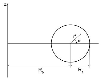
Figure 1: Cross-section of a torus by a half-plane  $\varphi = \text{const.}$
