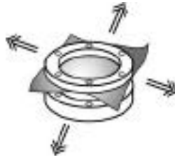
Figure 2. Schematic drawing of the stretcher assembly. Aluminized side of mylar faces the thicker ring.
