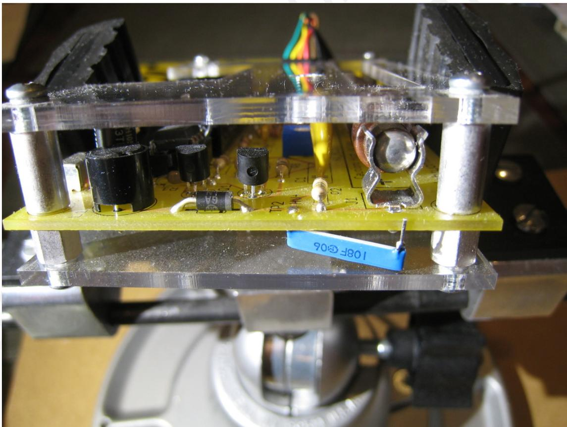
To measure the tube voltage, set the Plusivo meter to the  $2\text{ V DC}$  range, then place the positive probe on the unconnected lead of the  $1\text{ G}\Omega$  resistor, and the negative probe on the clip holding the far end of the Geiger tube. Figure out how to calculate the voltage at the HV+ test point from the meter reading. The tolerance of the  $1\text{ G}\Omega$  resistor is  $1\%$ , and the
