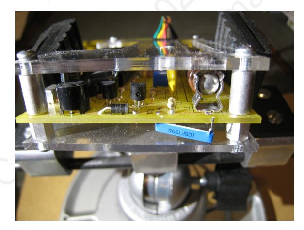
To measure the tube voltage, set a multimeter with 10 M $\Omega$  input impedance to measure DC volts, then place the positive probe on the unconnected lead of the 1 G $\Omega$  resistor, and the negative probe on the clip holding the far end of the Geiger tube. Figure out how to calculate the voltage at the HV+ test point from the meter reading. The tolerance of the
