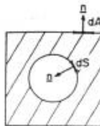
Fig. 1. Axial section of resonator through obstacle. The shaded area indicates the volume of the resonator.
