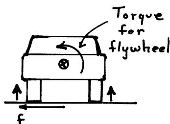
In the absence of the flywheel, the counterclockwise torque due to the normal forces at the wheels must oppose the clockwise torque due to the radial (transverse) friction force,  $f = Mv^2/r$ . With the flywheel, the normal forces exert no torque; so the flywheel must exert a clockwise torque  $= L_f$ , where  $L$  is the distance from the road to the center of mass. The counterclockwise torque  $L_f$  must be just sufficient to make the flywheel precess at the rate the car is turning.
