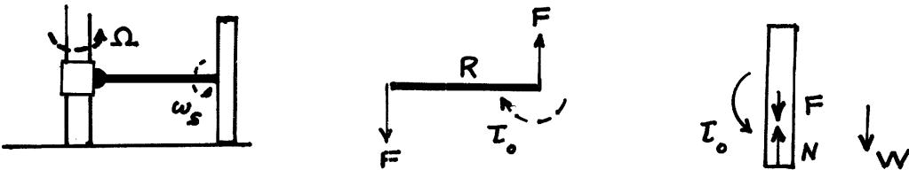
The axle exerts a torque  $T_o$  on the millstone and a vertical downward force  $F$ . The millstone exerts opposite force and torque on the axle. The coupling at the vertical column must also exert a downward force  $F$  on the axle.
