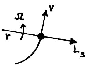
The torque due to the road is  $\tau = L_f = Mv^2 RL$
