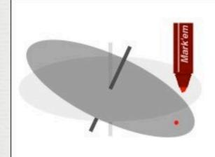
With the disc not spinning, we try the experiment. The disc changes orientation easily, as expected, and the red spot on the disc shows where it was pushed.
