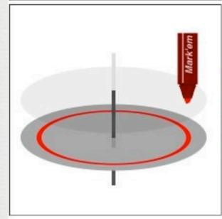
Now we do it with the disc rapidly spinning. As soon as the marker touches the disc, a red circle appears all the way around the disc. This red circle shows all the points where the disc is being pushed down. Naturally, no angular orientation change will occur when the disc is being pushed on all the points of a circular path which is centered on the disc. The whole disc will move down, just as you should expect it to move when you push it down on all points of the red circle!
