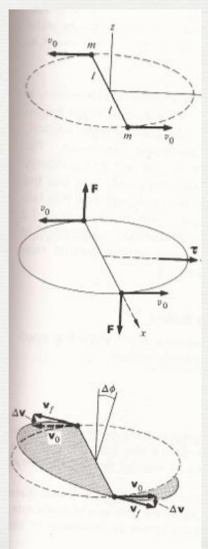
The motion of the particles causes the plane of rotation to tilt in a different direction from the applied force!
