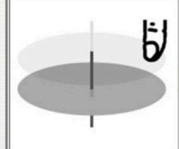
Now we get the disc spinning at a high rate, and do the same experiment again. This time the whole disc moves down, without changing orientation, even though we pushed it near the edge. How did it do that?
