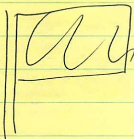
Flag flapping in wind. If flow was laminar, flag would lie on fixed position along streamlines. Instead, flag breaks flow into irregular pattern, and flaps along with it.
