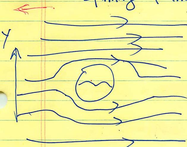
Symmetric wrt equator—no net force in  $y$  direction
