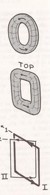
force on the top and bottom are opposite. The force on the pipe is the same as the force on the flywheel and that force is communicated to the suitcase. The top tilts to the right and the bottom to the left — as in sketch "D."
