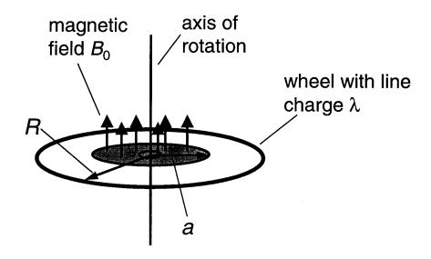
$$\int \vec{E} \cdot d\vec{l} = -\frac{d\vec{\Phi}}{dt} = \pi a^2 \frac{dB}{dt}, \text{ uniform} \Rightarrow E = \frac{\pi a^2 dB}{2\pi R} dt$$
