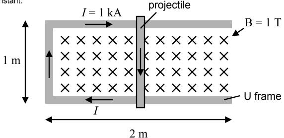
(a) Force is F = I B L, so acceleration is I B L/m. To move 1 m (= L) takes a time  $t_0 = (2L/a)^{1/2} = (2 m/I B)^{1/2}$ , so the velocity is  $v = a t_0 = (2 I B /m)^{1/2}L = (200)^{1/2}$  m/s = 14 m/s
