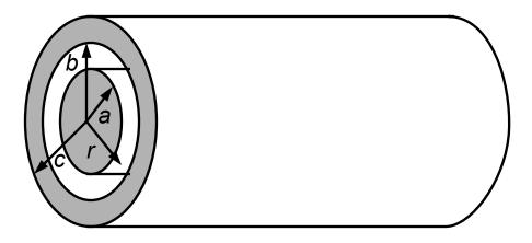
Use Ampere's law: In all cases, B points tangent to a circle centered on the axis of the cable, clockwise rotation in the schematic.
