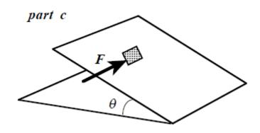
**Extra Credit:** A particle of mass m slides down an inclined plane under the influence of gravity. If the motion is resisted by a force  $f = kmv^2$ , show that the time required to move a distance d after starting from rest is
