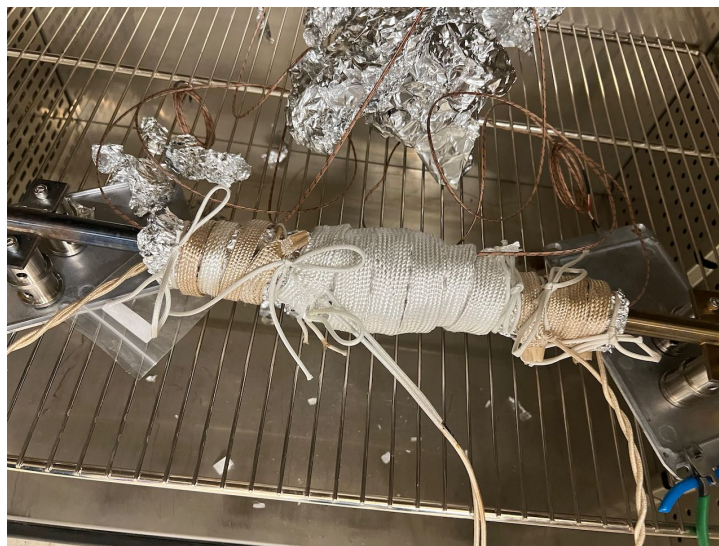
Figure 2.8: Heater tape wrapped around the spectroscopy cell before insulation was added. The central component of the heater tape was bleached white from being raised to high temperatures in a previous bake.
