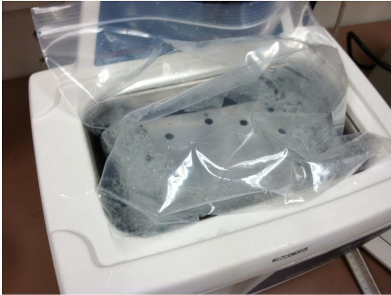
**Figure 2.16:** Photograph of sonication process using plastic bags to suspend the part.
