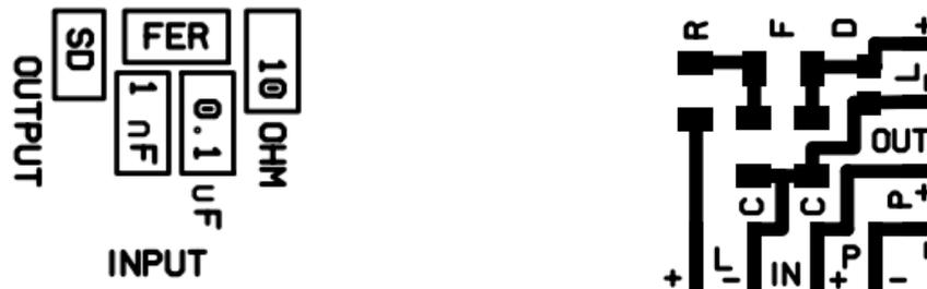
(a) printed circuit board components layout
