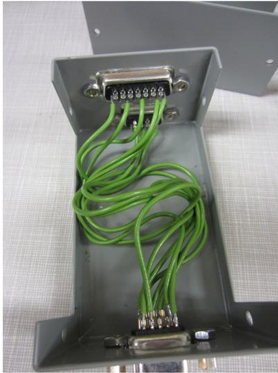
**Figure 2.13:** Wiring box; the wires connect the DB15HD to the DB15 and DB9 solder cup shells.
